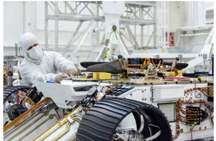
**An engineer works on attaching NASA's Mars Helicopter to the belly of the Mars 2020 rover — which has been flipped over for that purpose — on Aug. 28, 2019, at JPL. (NASA photo)**
