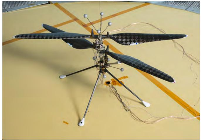
The demonstration vehicle used to prove that controlled and sustained flight is feasible in a Martian atmosphere. The first free flight of this prototype Mars Helicopter in atmospheric conditions similar to Mars occurred on May 31, 2016, in the JPL Space Simulator. (NASA photo)
