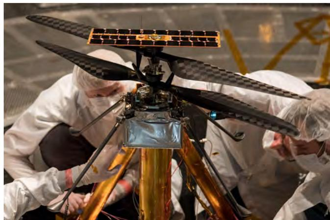
Members of NASA’s Mars Helicopter team prepare the flight model (the actual vehicle going to Mars) for a test in the JPL Space Simulator on Jan. 18, 2019. (NASA photo)
