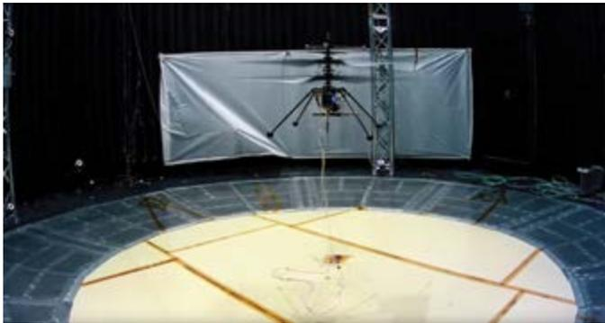
A subscale Mars Helicopter was tested in the NASA JPL vacuum chamber.
